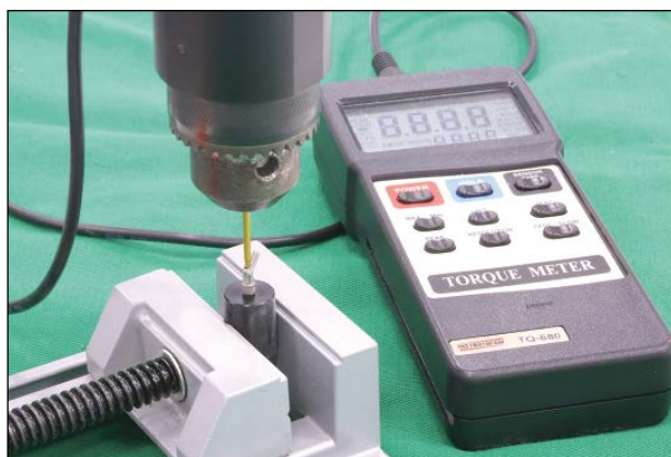
Fig 1 Digital prosthetic ratchet (TQ-680, Instrutherm) used to tighten the prosthetic abutments to the implants.
