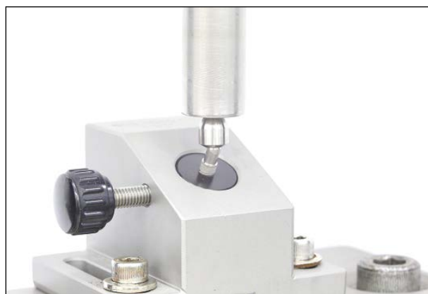
Fig 2 Static and dynamic loading: The hemispherical device is positioned on the abutment for application of vertical cyclic loads following ISO 14801:2007.
