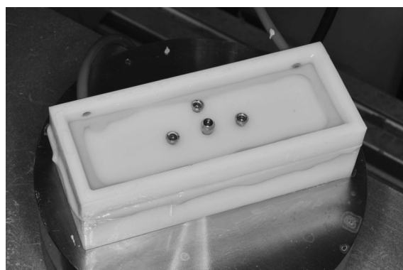
Figure 1 The artificial saliva bath unit controlled at 37 \pm 2^\circ\text{C} was set up for 5500 insertion-removal cycles.
