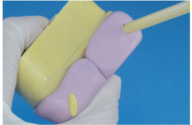
Figure 11. Inject polyvinyl siloxane cast material.
