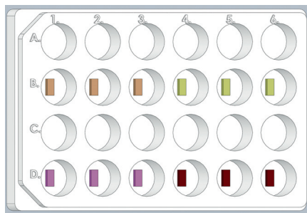
Figure 1. Experimental arrangement: 24-well cell culture flask with cement pellets, accounting for 10% of well surface area. All cement compositions tested in triplicate. Each color different cement composition.
