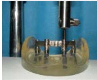
Fig 5 Implant reassembly with the framework attached permanently to the acrylic arch model.
