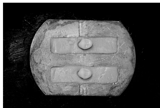
Figure 2 Silicone-acrylic tooth sets fabricated from the stainless steel mold.
