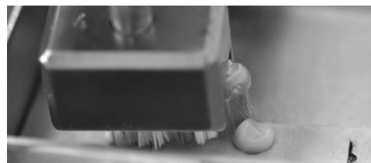
Figure 3 Silicone-acrylic tooth set positioned on the brushing machine.
