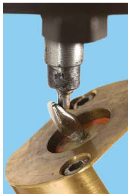
3 Assembled specimen being cyclically loaded at 30 degrees to long axis.
