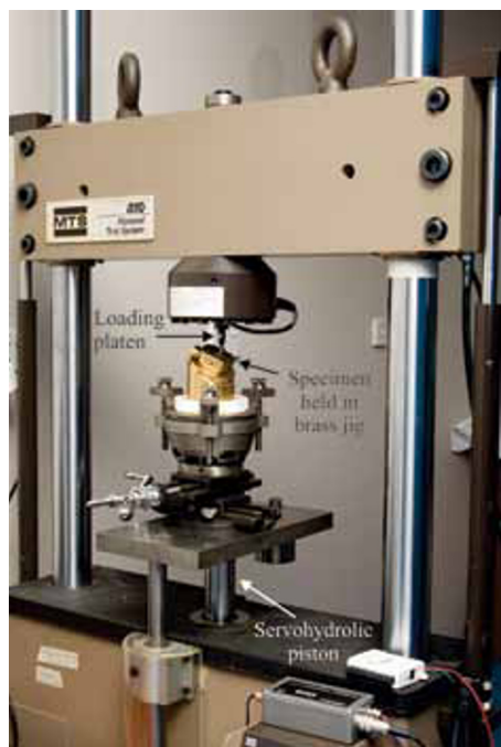
2 Assembled specimen fastened to adjustable (X-Y plane) customized device attached to servohydraulic machine.
