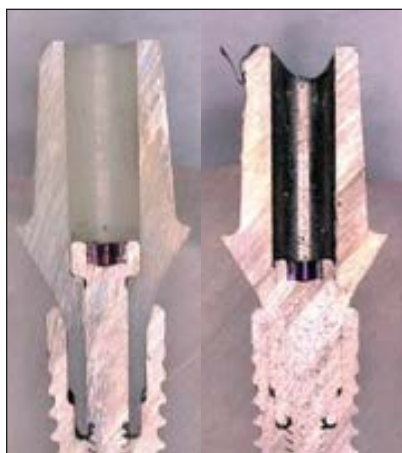
Fig 2 Longitudinally sectioned zirconium abutment/titanium implant and titanium abutment/titanium implant complexes.
