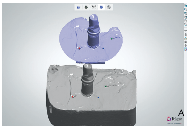
Figure 3. A, Software view of definitive abutment (blue). B, Software view of superimposed image with 3-point matching technique.
