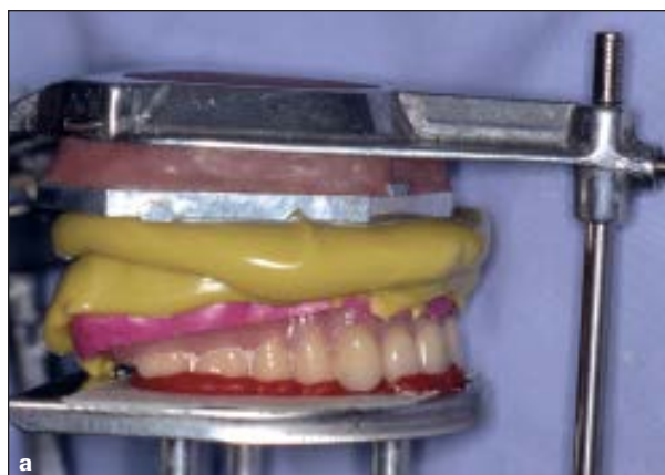
Fig 1 Measurements of the casts. (a) Semiadaptable articulator for cast calibration. (b) Elastomeric cast. (c) Optical targets for photogrammetric controls. (d) Block diagram of 3D measurement system.
