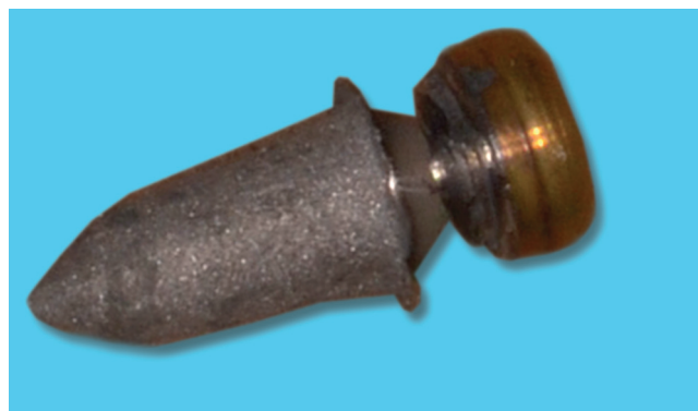
Figure 4. Laser welded Locator attachment.
