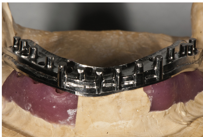
2 Digital design files interfaced with computer-controlled milling machines to produce precisely machined titanium frameworks.
