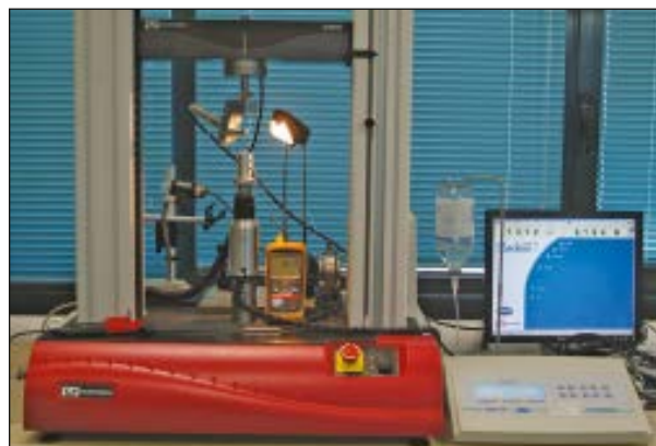
Fig 6 Test apparatus. (left) The Instron machine for electromechanic testing was used to apply a constant load on the contra-angle handpiece, the specimen, and the digital thermocouple thermometer; (right) the implant motor and the saline solution.
