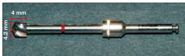
Fig 1 Test drill (4.2 Zero 1 Drill) used in the study. This drill design has a diameter of 4.2 mm and a cutting surface length of 4 mm. The sharpening of the cutting edge was similar to that of a pilot drill.
