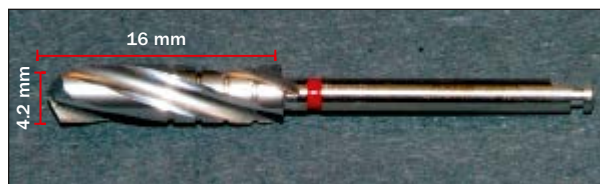
Fig 2 Control drill (4.2 Twist Standard Drill). This standard drill design has a diameter of 4.2 mm and a cutting surface length of 16 mm. The cutting edges were designed to exclusively increase the diameter of the site being drilled.
