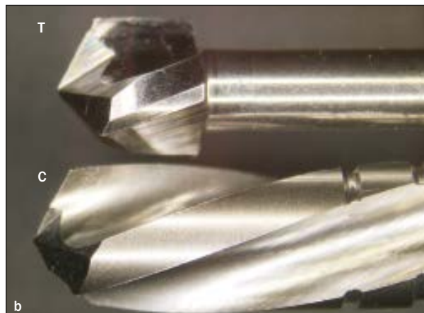
Fig 3 High-magnification images of the evaluated implant drills: T (test), 4.2 Zero 1 Drill; C (control), 4.2 Twist Standard Drill. (a) View from the top; (b) lateral view.
