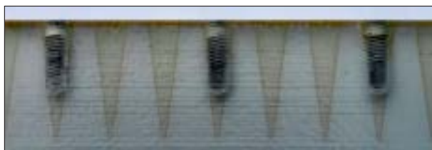
Fig 3 (below) Resin block with the implants in place.
