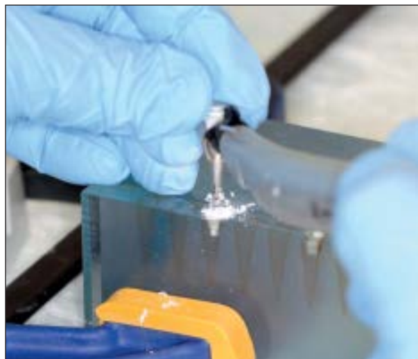
Fig 1 (above) The 12 × 2 × 8-mm resin block with nine pilot holes drilled 1 inch apart.
