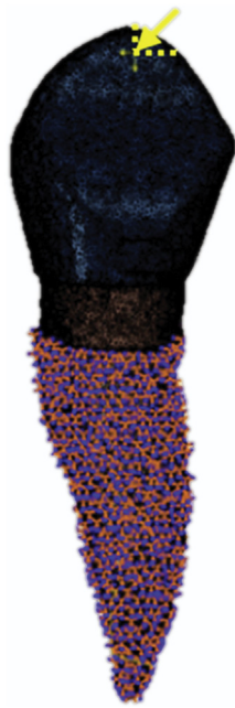
Figure 3. Three-dimensional virtual image representing boundary conditions, loading, and finite element mesh. Yellow arrow indicates loading area, and periodontal ligament shows boundary conditions of model.
