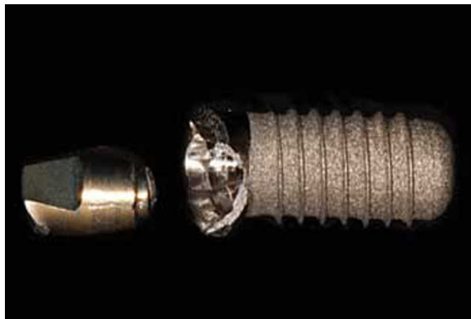
8 Fracture of collar wall and head of screw just below base of cone in abutment.
