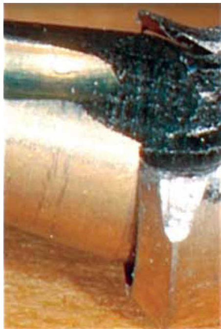
3 Failed specimen after fatigue loading due to presence of space between abutment and implant.
