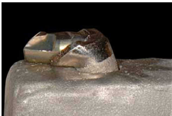
4 Failed specimen after application of vertical compressive load.
