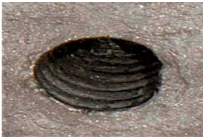
1 Integrity of implant threads formed by implant when metal mold was fabricated. Integrity was needed to allow screwing and unscrewing of tested implants.
