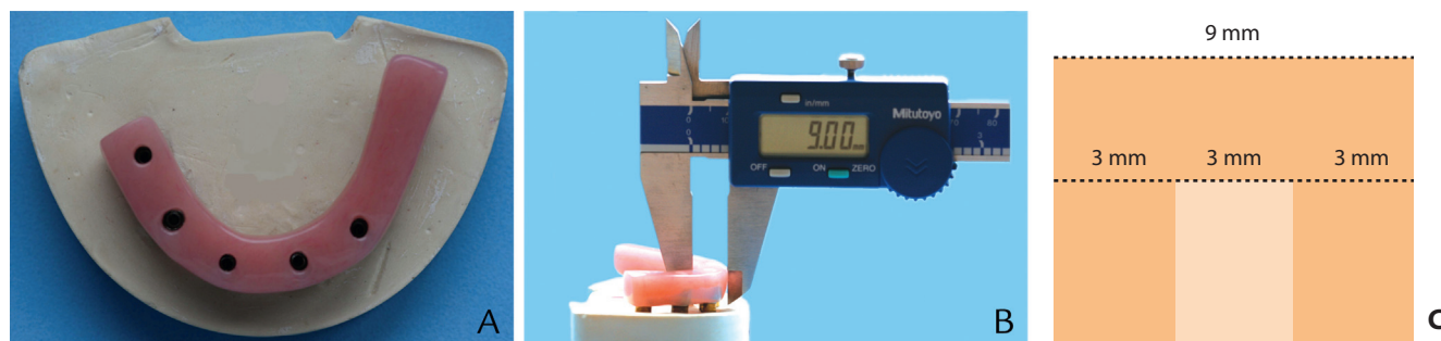
Figure 2. Veneer. A, Occlusal view. B, Thickness measurement. C, Transverse section.
